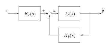
Figure 12: 2-DOF with PID
