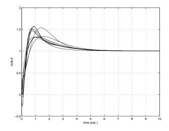
Figure 9: step response with nonsmooth PID controller
