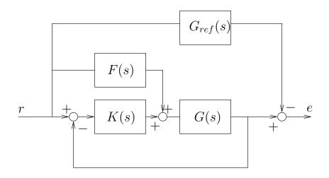
Figure 5: feedforward design with reference model
