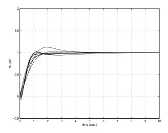
Figure 10: step response with PID + feedforward control, slow reference model
