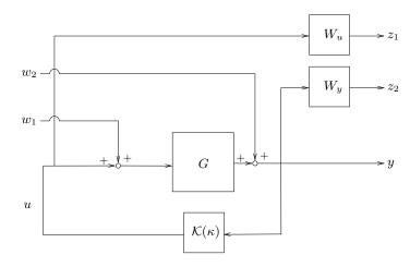
Figure 3: observer-based feedback with augmented model
