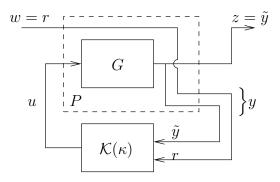
Figure 13: Equivalent standard form to 2-DOF with PID
