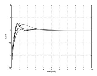
Figure 11: step response with PID + feedforward control, fast reference model
