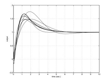
Figure 7: step response with robust controller
