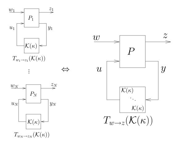
Figure 4: reliable control based on N scenarios
