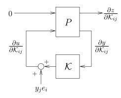
Figure 2: interconnection for gradient computation
